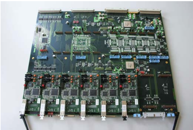
Fig. 6. Implementation platform: the TOM-board (Timing Output Module), with 8 FPGAs from Altera’s Stratix-family
