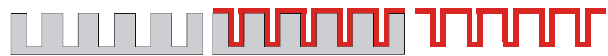
Figure 1. Moulding of a SiRN hair: etching holes in silicon, covering by SiRN and finally removing silicon.
