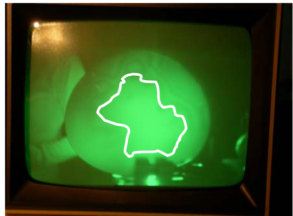
Fig. 7. 30 nm thick SiN layers on high bow wafers bonding. The bow affect the bonding as less than 40 % is bonded (inside the white line).
