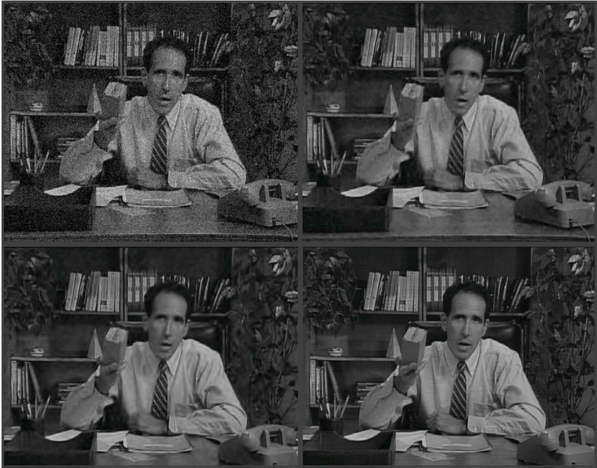
Fig. 4. (a) Noisy 24-th frame of the salesman sequence \sigma = 15 . (b) Resulting frame after filtering with SEQWT filter. (c) Resulting frame after filtering with proposed filter. (d) Noise-free frame
