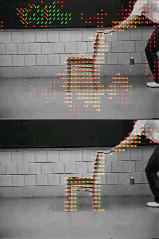
Fig. 2. Motion field for 15-th frame of 'chair' sequence, before and after filtering.
