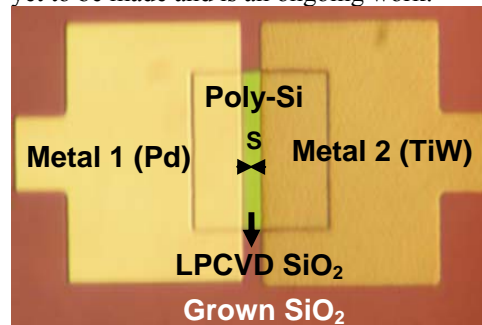
Fig.9 shows the microscope image of a fabricated CP device.
