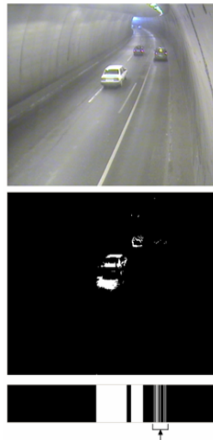
Figure 1. (a) Top: An input image from a tunnel. There is a static vehicle in the most right lane. (b) Middle: The corresponding thresholded single frame difference (TSFD) image. (c) Bottom: The resulting scan line. The areas designated by the arrow are discarded due to the minimum width constraint.
