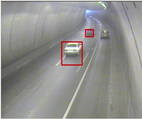
Figure 4. The result of our object detection algorithm on the frame from Figure 1. The moving vehicles are detected and the static vehicle is not detected.
