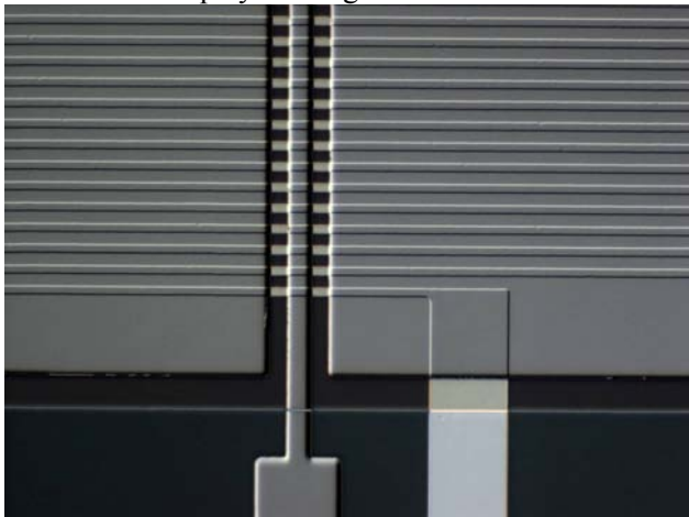
Figure 13 Micrograph of the outer area of an 25 turn, 5 μm pitch coil with inner diameter 125 μm. Spiral = 45 nm Al, insulation 130 nm SiO, washer and return 180 nm Nb. Nominal value of L = 123 nH.
