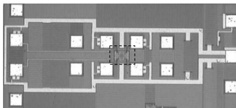
Fig. 4. Chip micrograph of the proposed ILFD
