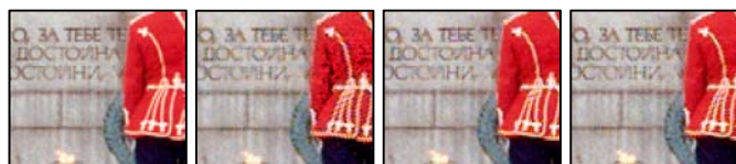
Fig. 11. Aliasing and “corrode” effect – From left-to-right: (a) – ROI on test image 14 ; (b) – SHTI in logarithmic exposure space; (c) – Laroche-Prescott; (d) – Hamilton-Adams interpolations.
