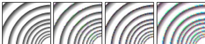
Fig. 7. From left-to-right: (a) – ROI on test image 1 ; (b) – SHTI in logarithmic space; (c) – Hamilton-Adams; (d) – pattern recognition interpolations.
