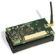
Figure 1: Mica2 sensor node [5]
