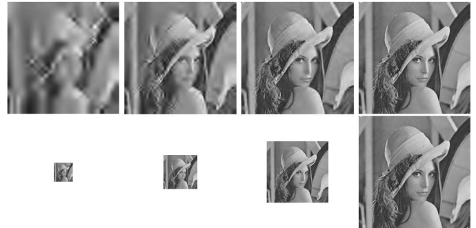
Fig. 1. Scalability in quality (above) and in resolution (below) applied to the Lena image.
