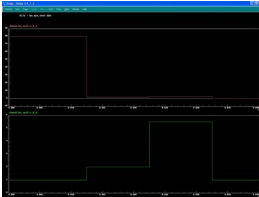
Figure 4. VHDL-AMS simulation input ( \epsilon_r and t_{ox} ) in the case of a bare Au electrode, functionalization, DNA hybridization and failure.
