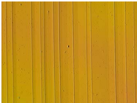
Fig. 11: the cracks on the silicon oxide under the tensile loading.
