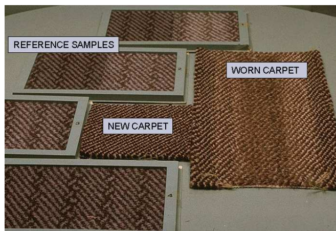
Fig. 1. Test environment used by human expert to classify wear carpets. Source: Textile Department, Ghent University
