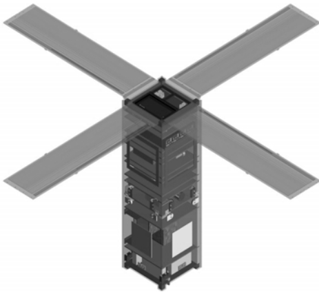
Fig. 3. The planned successor of DelfiC3: Delfi-n3Xt. The dimensions are also 10x10x30cm. It is equipped a Delfi-C3 like VHF antenna system with deployable antennas 50cm for both transmission in the VHF band and reception in the UHF band. Also the OLFAR experiment will make use of these antennas. Delfi-n3Xt has attitude control and is sun pointing.
