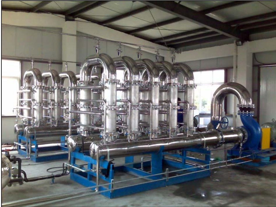
InoCep™ micro-filtration system for product recovery
