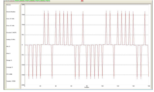
Fig. 9. The ADC samples of the UWB signal generated by AWG
